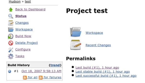
If you click that, you can see the status of all the tasks. You can schedule the execution of a task from here, too. Task executions are numbered like "123-456" where 123 portion refers to the latest build and 456 portion refers to the sequential number (so that you can execute a task multiple times with the same build.) The build number portion is significant because when a batch task runs, it sees the workspace as of the result of this build.
