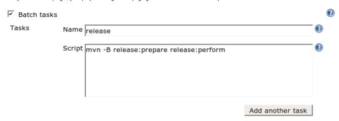
A batch task consists of a shell script and a name. When you execute a build, the shell script gets run on the workspace, just like a build. Batch tasks and builds "lock" the workspace, so when one of those activities is in progress, all the others will block in the queue.
