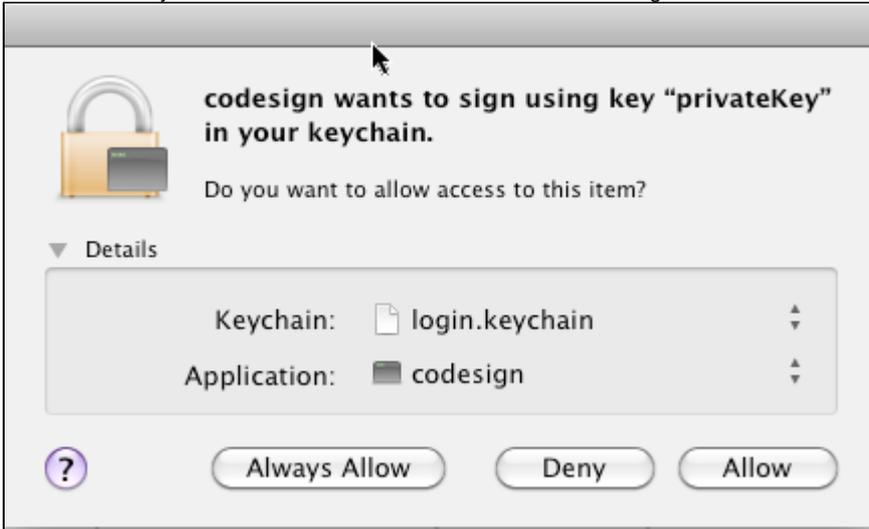
If this prompt is not showing on the build machine, you can force it to appear by running the codesign command that failed from a terminal on the build machine: `/usr/bin/codesign --force --sign "iPhone Distribution: .....`
